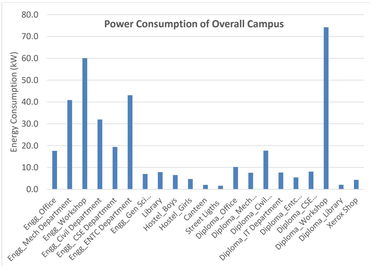
Fig.3.1 Total Power Consumption of Different Units
