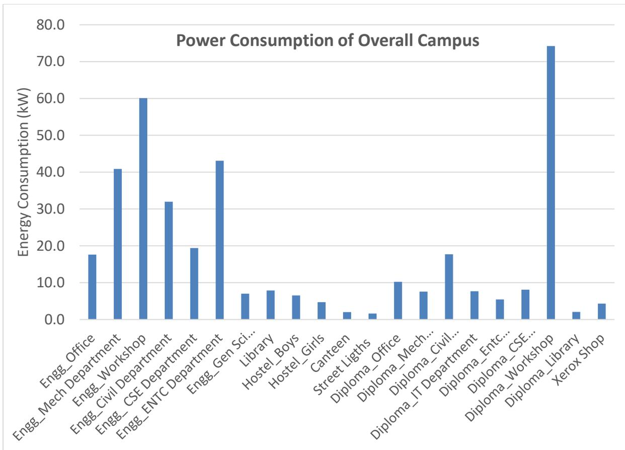
Fig.3.1 Total Power Consumption of Different Units
